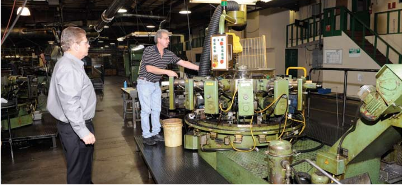
ABOVE: John Griner, left, with plant manager, John Elmore, operating a Hydromat rotary transfer machine with robotic loading that machines cold formed, starter parts for the automotive industry.
